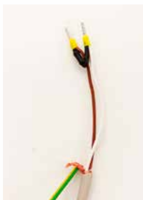
④ Green/yellow shield ground connection
