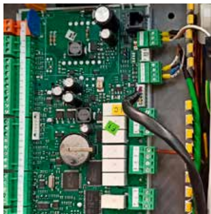
⑥a \mu PC Plan connection
