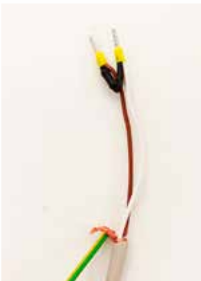
4 Green/yellow shield ground connection
