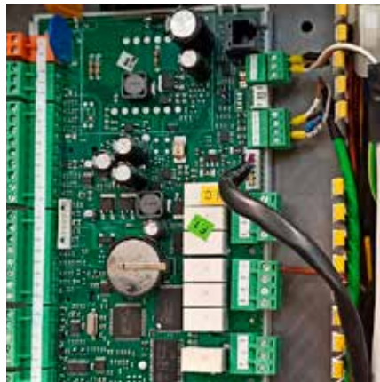
⑥a \mu PC PLan connection
