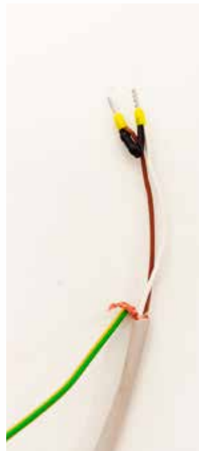
③ Green/yellow shield ground connection
