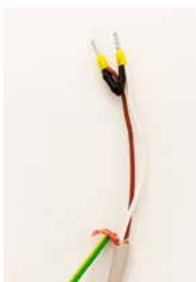
④ Green/yellow shield ground connection
