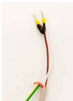
④ Green/yellow shield ground connection
