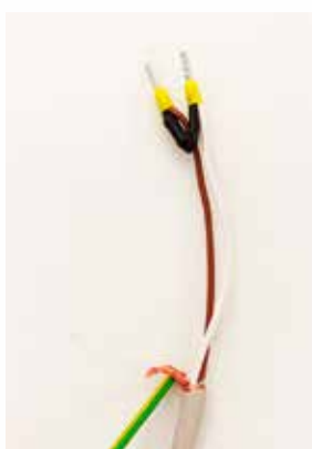
④ Green/yellow shield ground connection
